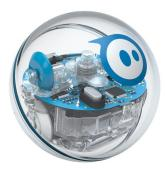
Sphero is a spherical robot. It is the size of a tennis ball connected via bluetooth to a mobile device. The Sphero can be used to transform teaching and learning across various curriculum areas. Students can code them to roll around the school using space, shape and measurement maths or dance an Irish jig.
